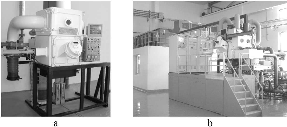
Fig. 9 Laboratory (a) and production (b) units for material evaporation and condensation in vacuum
